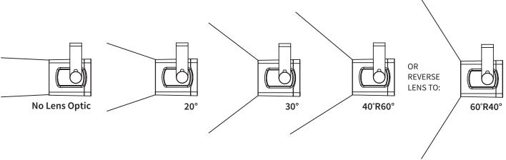
To add or change an OPTI-SCULPT lens, unscrew the thumbscrews from the front panel and remove the acrylic panel. Install the desired OPTI-SCULPT onto the posts. Place the acrylic panel on top and re-secure it with the four thumbscrews.
