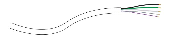
Purple and Gray wires are to be used with standard 0-10V dimmers. These wires should be properly insulated from all electrical circuits when not used.
