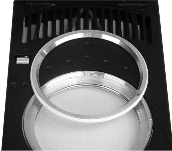
2. Once the Threaded Collars are removed, insert a B size gobo so that it lays flat against the gobo wheel.
