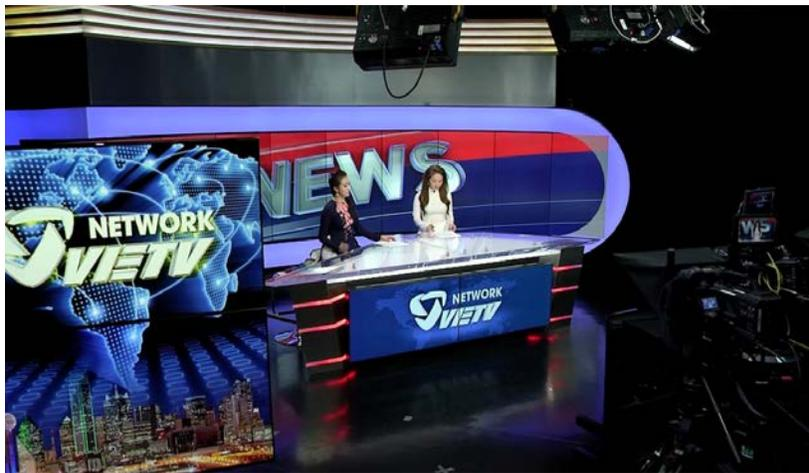
John also reported how much brighter the RoscoLED Tape was than the product he used in the Dallas studio. He ended up using half as much LED tape in the Houston studio than he did last time. The U-shaped band in Dallas, for example, necessitated 2-3 strips of LED tape. John was able to get the same light level with just one strip of RoscoLED Tape centered in the middle of the 11" high band. This left John with extra RoscoLED Tape Kits, which he already has plans to install in another studio.
