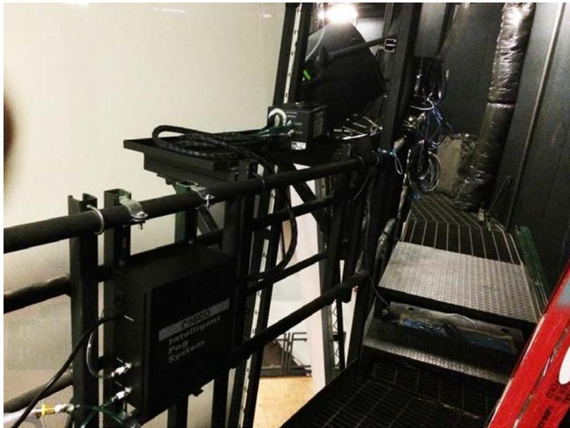
The Rosco Intelligent Fog System provided a long-term fog and haze solution for the Manufacturing Innovation Theatre. Its self-cleaning functionality, modular components and its centralized fluid delivery system were all desirable features for this permanent fog-generating installation.
